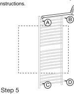
Install the tube onto the wall support (4)
