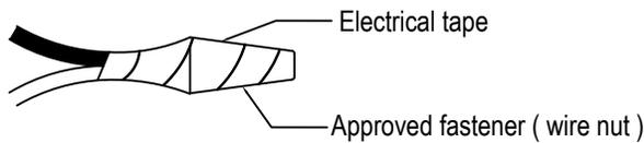
6. Connect the black fixture lead to the black wire in the outlet box. Fasten the joined wires as in step 6.
