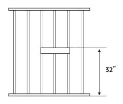
To properly support the weight of the vanity and countersink, secure to stud framing or 2x6 bracing behind the finished wall.
