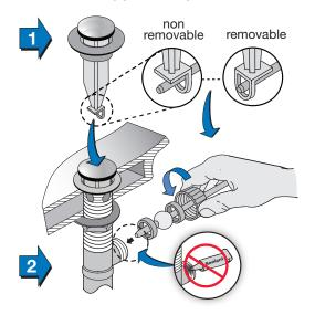
Step 7 Connect lift rod and adjust linkage
