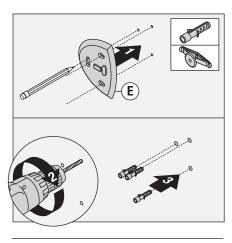
Place mounting plate (E) in position, mark and drill 1/8" pilot holes into stud.
