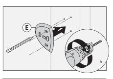
Remove cover of hand shower cradle (C). Install cradle and mounting plate (E). Secure with three screws (D). Replace cover on hand shower cradle.
