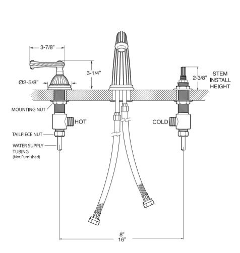
**NOTE:** Spout and valves install through 1-1/4" diameter holes
