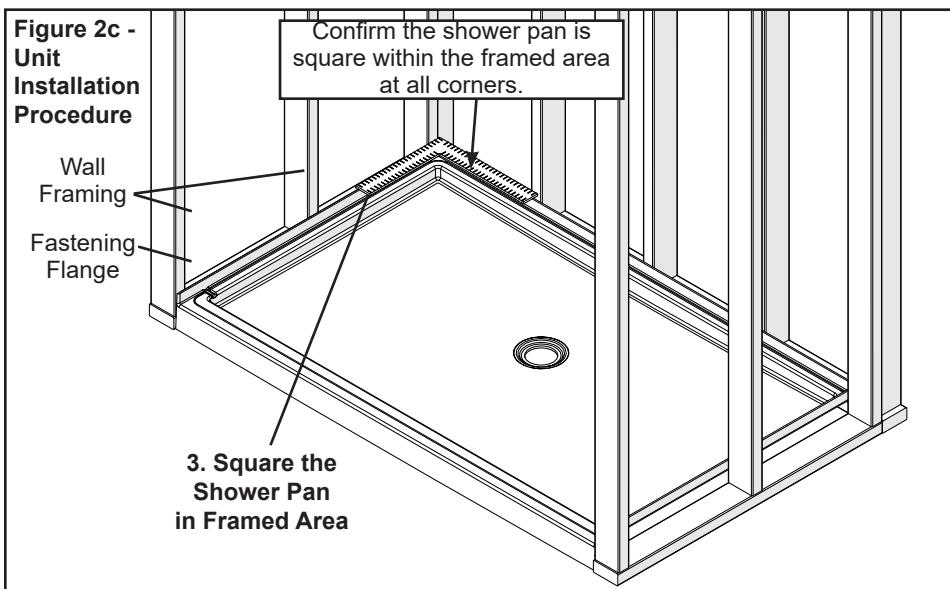
**CAUTION:** It is advisable to protect the unit surface with a thin plywood or cardboard shield while fastening the flange to the framing.
