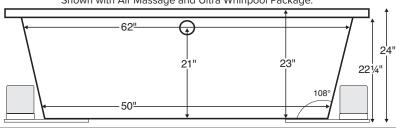
IMPORTANT: Air baths and tubs with a pre-leveled foam base add 2-3" to overall tub height.
