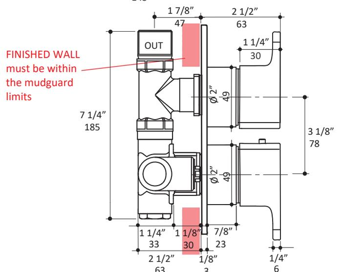
LACAVA reserves the right to revise any dimension or information on this sheet without notice. Dimensions are nominal and may vary within an industry accepted tolerance of 1/4". Drawings provided herein are meant to give the user an idea of the product and are not made to scale. Location of plumbing is meant for reference, your specific application may vary. Revised: 03/29/2019
