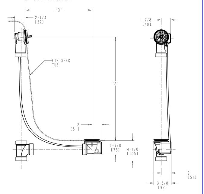
DIMENSIONS ARE IN INCHES AND [MILLIMETERS].
