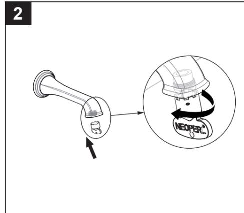
Remove tub spout flow guide with key and flush out debris.
