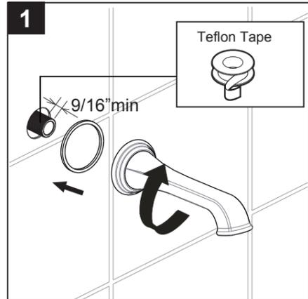
Apply teflon tape to the tub spout nipple and thread on wall tub spout.
