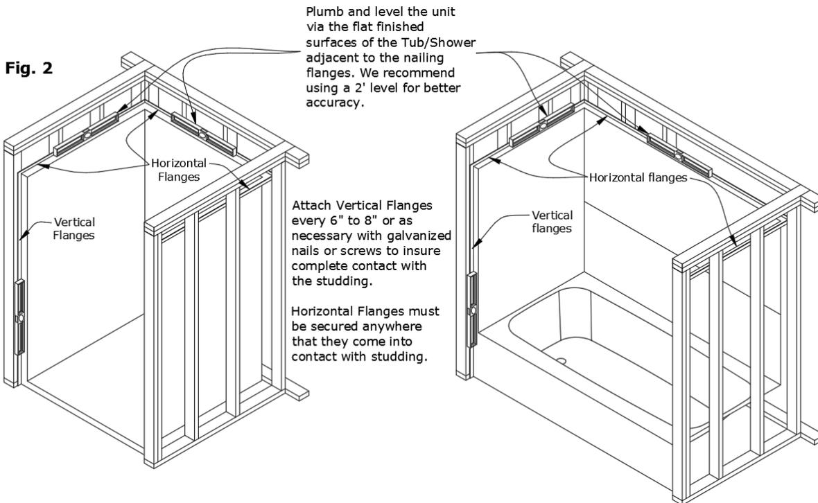
*(In an application where the unit is installed over wall board, the Clarion Bathware E-Z Wall Trim Kit (Fig 3) will help you finish your installation quick and easy. For best results your fasteners will need to be flush with the nailing flange. Clarion Bathware recommends centering and counter sinking a corrosion resistance fastener on the nailing flange. Raised fasteners will result in a problematic finishing process of the trim kit.)*
