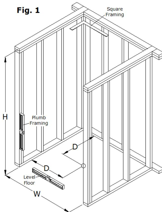
\* H= Height of framing pocket should be at least the height of unit that is being installed.
