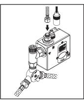
(5) Connect hose and sensor plug from faucet to control module. (Note: Do not connect sensor cables when hands are wet.)
