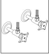
(4) Connect inlet hoses to angle stops.
