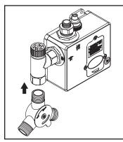
(2) Secure mixing valve onto (3) Secure inlet hoses to the control module as shown mixing valve as shown in in picture. (Note: Not for -LM picture. (Note: Not for -LM variations.)
