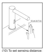
Press and hold ON/OFF button for 5 ~ 7 seconds. When the LED sensor light remains lit, the system has entered setup mode. Place an object, or your hand, at desired distance. Note that the LED sensor light should be flashing when object is detected. To set the new distance, press the ON/OFF button again, your settings have been saved.
