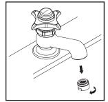
(4) Important: For model# 0255-AX, after installation is complete, remove aerator. Turn on water supply and turn on handle to allow water to run at least one minute. While water is running, check for leaks. Turn off handle and replace aerator.
