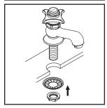
(2) Apply a layer of plumbers putty to underside of faucet, place faucet shank through the mounting hole. Slide the crowfoot washer through shank from underneath of the sink. Tighten the locknut with the help of a 1-3/32" socket.
