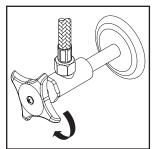
(1) Shut off water supply. Remove old faucet. Clean mounting surface in preparation for new faucet.
