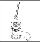
(6) Use wrench to adjust brass square nut, turn counterclockwise to tighten the cartridge and turn it clockwise to loosen the cartridge until the faucet functions properly then proceed to tighten the cartridge 90° more before reassembling the Celcon Samson nut, sleeve, and handle cap back in place.
