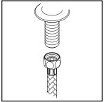
(3) When using stainless steel braided faucet supply hose; this faucet requires on end of the supply hose to have 1/2" female IPS connection. The other end of this supply hose must match the thread on the water supply valve under the sink. Once you've identified the required size, carefully follow the manufacturer's installation instruction to install hose.
