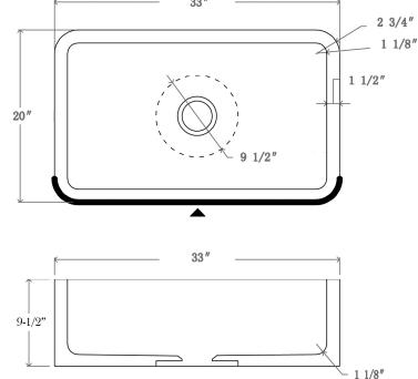
Dimensions of fixture are nominal and may vary within the range of tolerances established by ANSI Standard A112.19.2. Dimensions and specifications subject to change without notice.
