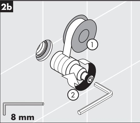
Wrap the mounting piece with Teflon tape.
