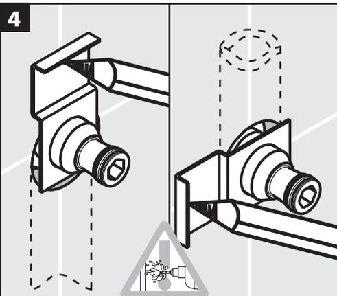
Position the support over the mounting piece.
