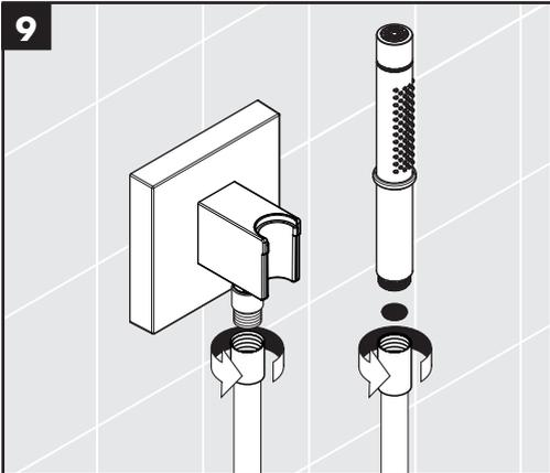
Place a rubber washer in the short end of the handshower hose. Connect this end to the outlet.
