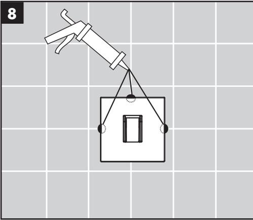
Place a small dab of sealant at the top and side grout joints.
